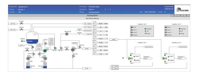
Technical data from the CIP equipment's PLC is collected every second, 24/7, which is saved, structured and presented in various reports – using the Win10 computer.
