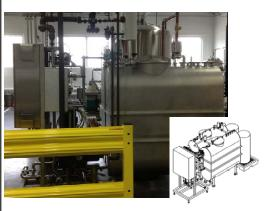
The MEC-FX series CIP cleaning equipment is specifically designed to address the challenges and issues associated with cleaning brew house skids (mashtun, brew kettles, whirlpools), fermenters, storage tanks and transfer lines within small to medium sized breweries.
